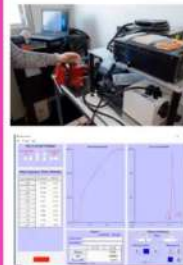
Skin Carotenoid Resonance Raman Spectroscopy
